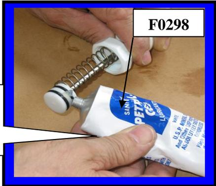
Installing **Plunger Assembly** into Faucet body
