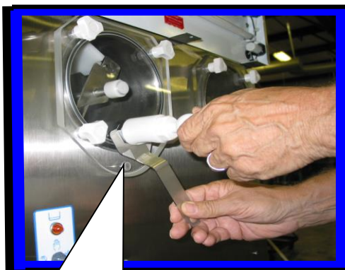
Align Faucet Assembly opening to bottom of faceplate then tighten nut
