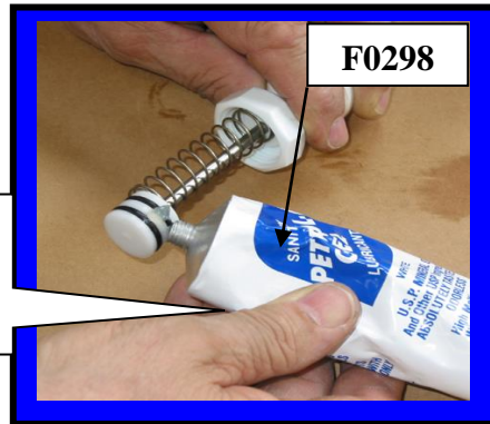
Lubricating O-rings with Petro-Gel
