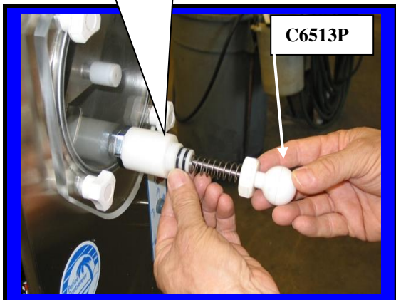
Installing Plunger Assembly into Faucet body
