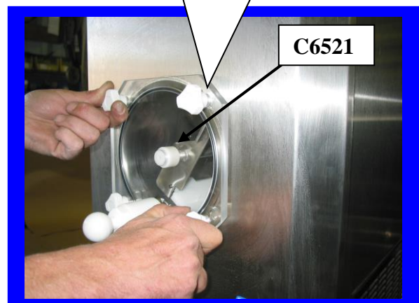
Installing small Faceplate onto front of Machine.
