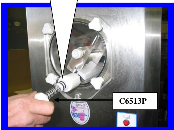
Installing Plunger Assembly into Faucet body
