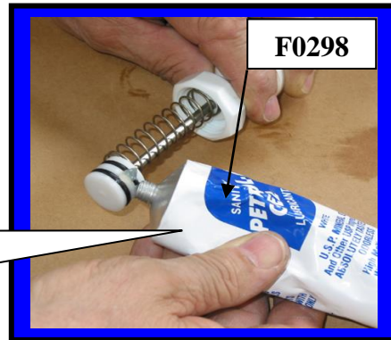
Install O-rings onto plunger
