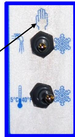
**Off** - The hand symbol is the recognized international symbol for "stop". In this position, the machine will not run.
