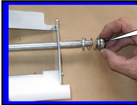
Step 5: Install spring seal F0355
