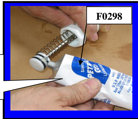
Lubricating O-rings with Petro-Gel
