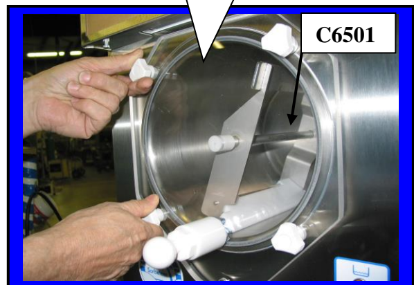
Installing large Faceplate onto front of Machine.
