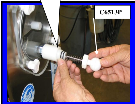
Installing Plunger Assembly into Faucet body
