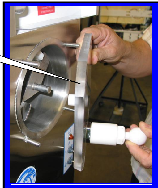
Installing faceplate C6521 onto front of Machine.
