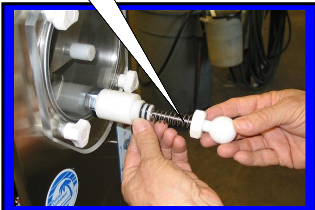
Installing faceplate C6521 onto front of Machine.
