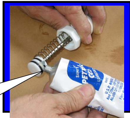
Installing O-rings onto plunger F 0491
