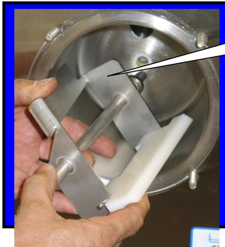
Step 7: Install beater bar C6519 into cylinder.
