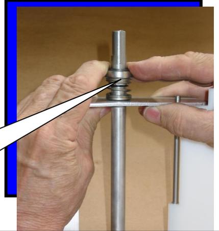
Step 6: Squeeze and release spring. Be sure the spring returns to normal before installing into machine.
