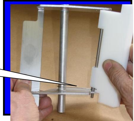
Step 2: Insert rod end into beater bar frame.
