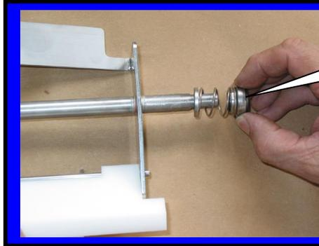
Step 5: Install spring seal F0355
