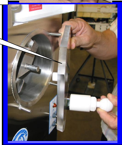
Install faceplate C6521 onto front of Machine.
