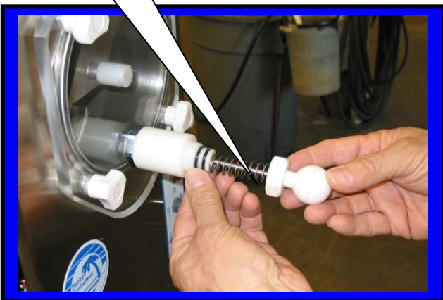
Install plunger assembly C6513P into faucet body
