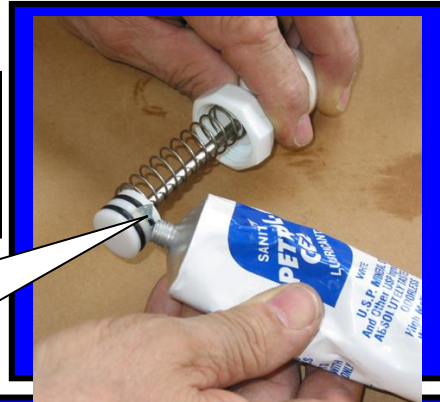
Install o-rings F0491 onto plunger
